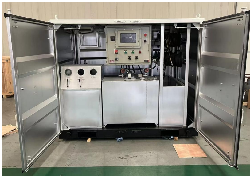
Hydraulic control unit
