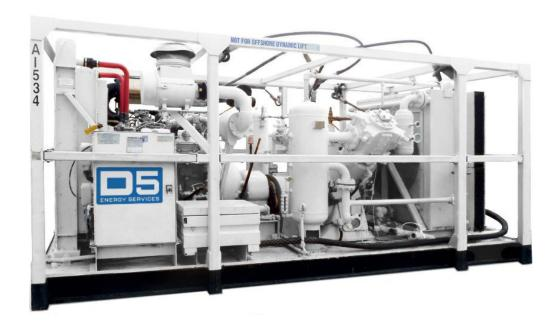
D5 Energy Services uses the latest Joy WB-12 booster design for all its booster compressors. These units boost the air from the compressors (or from the Membrane Nitrogen Generation Units) to the output pressures required, and will under ideal circumstances boost to a maximum continuous output pressure of 2500 psi.
