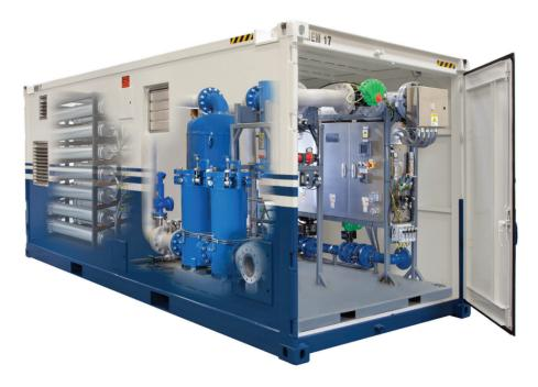
Compressed air from feed-air screw compressors is delivered to the common manifold for delivery to the membrane bundles in the membrane package. Bundles are composed of millions of polymer-based hair-fine tubes. Because they are so small, it is critical that moisture, dust, dirt particles, and trace oil vapours be removed prior to processing to protect the membranes. A sophisticated filtration system is included in the membrane skid package.
